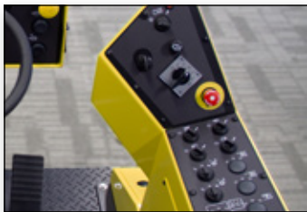
Jack and machine lighting controls
